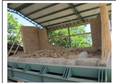
Photo 4 Tiltable test of the adobe masonry walls (UES)
