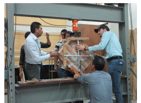
Photo 3 The direct shear test of masonry walls (UES)
